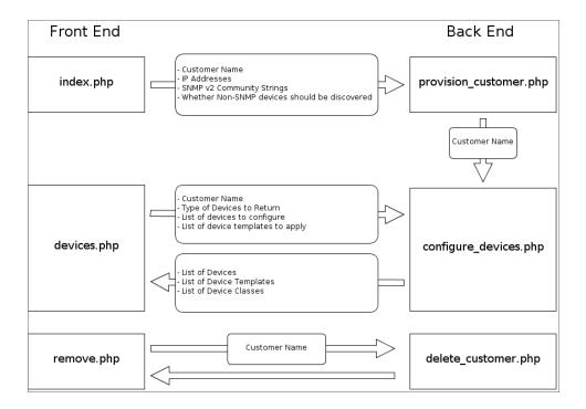
When a back-end procedure is unsuccessful, an error message is returned to the appropriate front-end page.
