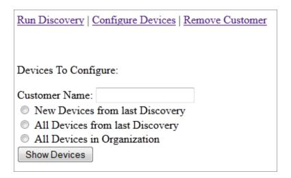
When you enter a customer name and select the [Show Devices] button, the configure\_devices.php script returns a list of devices that are then displayed in the devices.php page. For each device in the list of devices, the devices.php page displays a drop-down list of all device templates in the Service Level column. The last device template that was applied to the device is selected by default:
