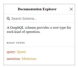
When you click one of the root operation types, a list of objects that are available for that operation type displays. Each object lists the object name, the arguments that can be passed into that object, the object's return type, and a definition of that object.
