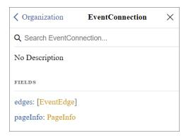
13. EventConnection is a connection type. Connection types consist of one or more edges that connect two nodes. The schema reflects this, so from EventConnection, click [EventEdge]:
