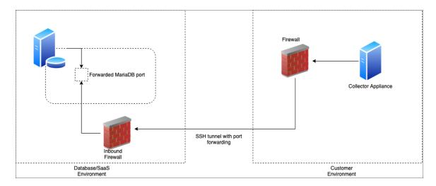
The benefits of this method are that no ingress firewall rules need to be added, as the collector initiates an outbound connection, and no new TCP ports are opened on the network that contains the Data Collectors.
