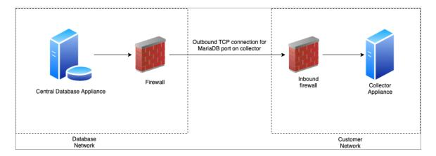
The benefit of the traditional method is that communication to the Database Server is extremely limited, so the Database Server remains as secure as possible.
