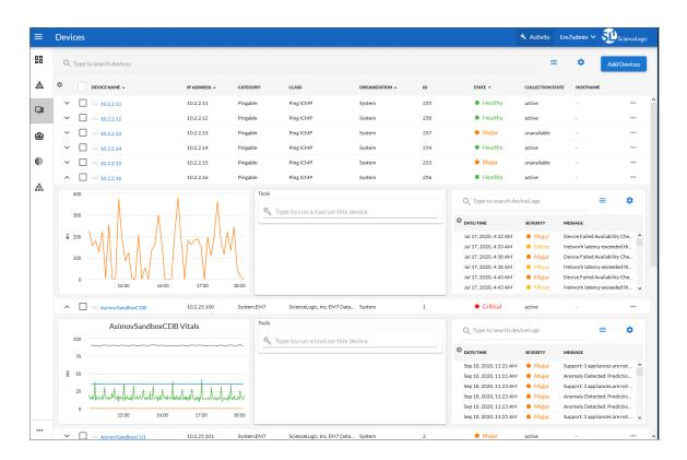
SL1 allows you to monitor and manage hardware and applications within your network. SL1 provides a networkwide view through a "single pane of glass." This means that you can monitor status, create policies, define thresholds, and receive notifications, all through a single, browser-based application.
