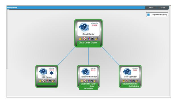
• The **Device Components** page (Registry > Devices > Device Components) displays a list of all root devices and component devices discovered by SL1 in an indented view, so you can easily view the hierarchy and relationships between child devices, parent devices, and root devices. To view the component devices associated with CloudCenter Suite, find the CloudCenter Suite root device and click its plus icon (+):
