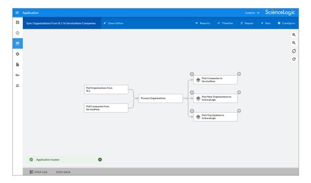
The **Application** detail page contains the logic for the application. In the main viewing pane, the steps for the application are organized as a flowchart. Each rectangular block is a step, and the arrows indicate the order in which the steps will execute when you run the application. The color of each step changes to show the progress of the application run as it runs: green for success, red for failure, and blue for running.
