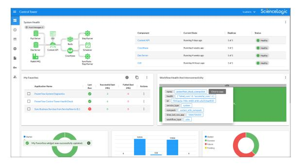
The PowerFlow Control Tower page contains the System Health, the Favorite Applications, and the Workflow Health and Interconnectivity widgets alongside high-level statistics about the health of the worker services that are being used by the PowerFlow instance.
