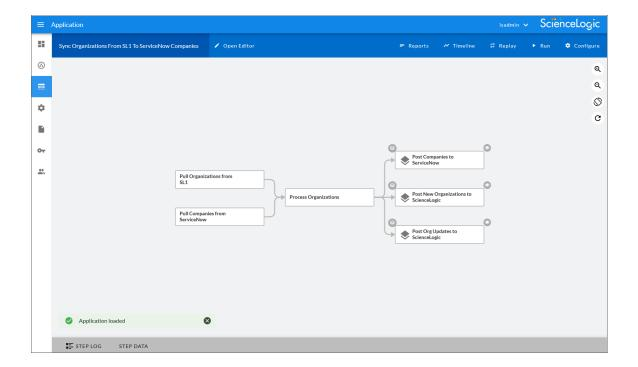
PowerFlow application JSON objects are defined by configuration settings, steps that make up the application, and application-wide variables used as parameters for each step. The parameters of each step can be configured dynamically, and each step can be named uniquely while still sharing the same underlying class, allowing for maximum re-use of code.
