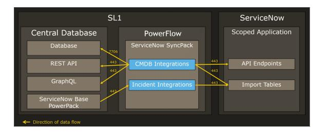
The workflow includes the following components and their communication methods:
